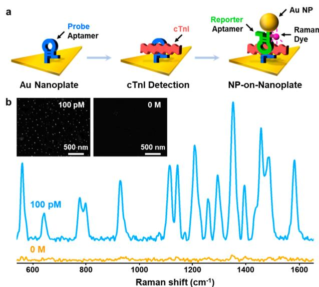
**Figure 1.** (a) Schematic representation of the cardiac troponin I protein (cTnI) detection procedure using an aptamer-immobilized Au nanoplate. (b) Surface-enhanced Raman scattering (SERS) spectra of Cy5 measured from Au nanoparticles (NPs)-on-nanoplate structure after detection of cTnI (100 pM, blue spectrum) and the control sample (orange spectrum). The inset shows SEM images of Au NPs-on-nanoplate structures after detection of cTnI (left panel) and the control sample (right panel).
