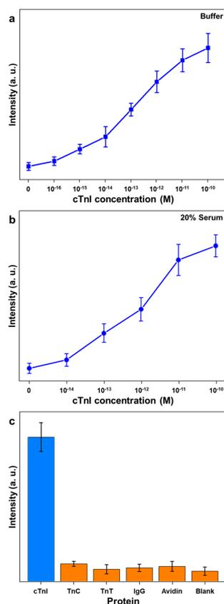
**Figure 3.** (a) Plot of  $1580\text{ cm}^{-1}$  band intensity versus cTnI concentration (0– $10^{-10}$  M) in buffer. (b) Plot of  $1580\text{ cm}^{-1}$  band intensity versus cTnI concentration (0– $10^{-10}$  M) in 20% serum. (c) Plot of  $1580\text{ cm}^{-1}$  band intensity versus proteins (cTnI, TnC, TnT, IgG, avidin, and control sample). The data represent the average plus standard deviation from ten measurements.
