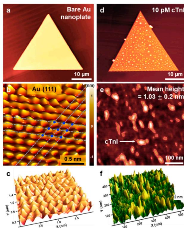
**Figure 2.** (a) Atomic force microscopy (AFM) topography image of a bare Au nanoplate. (b) Fourier bandpass-filtered atomic stick-slip image showing a well-defined Au (111) surface. (c) Three-dimensional Fourier bandpass-filtered atomic stick-slip image of the Au (111) surface. (d) AFM topography image of an aptamer-immobilized Au nanoplate after reaction with cTnI (10 pM). (e) Magnified and (f) three-dimensional AFM images of a cTnI-captured Au nanoplate.
