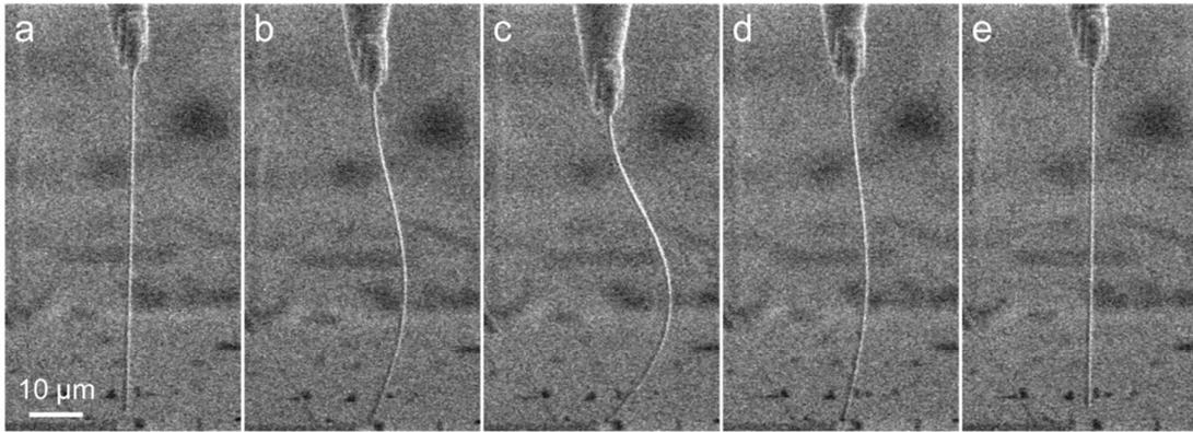
**Figure S5.** SEM images showing the flexible bending and recovery of a Au NW nanoinjector as it is pushed against a solid surface.
