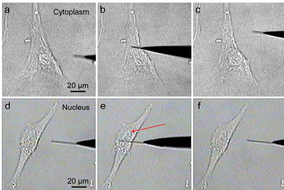
**Figure S1.** Optical images of SK-N-SH cells before (a,d), during (b,e), and after (c,f) insertion of Au NW nanoinjectors into the cytoplasm (a-c) or nucleus (d-f) of the cells. The red arrow in (e) denotes a nuclear membrane.
