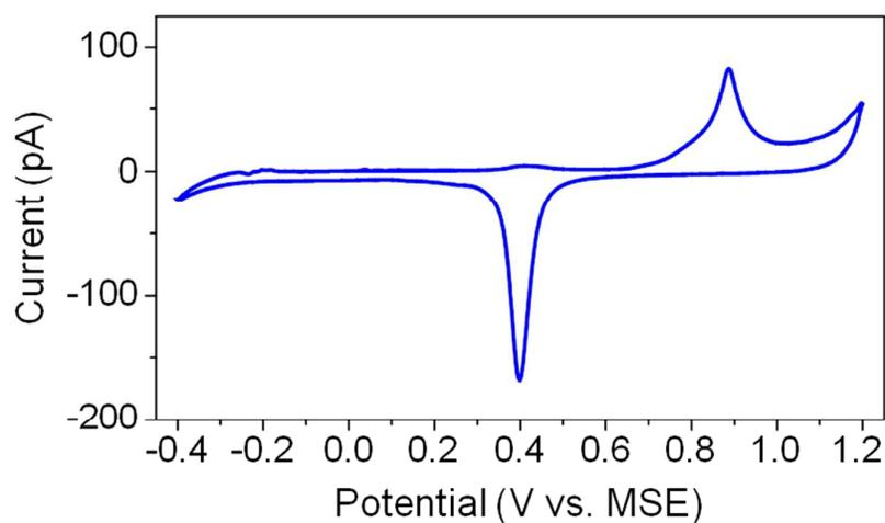
**Figure S4.** Cyclic voltammogram of a Au NW in a 50 mM sulfuric acid solution. Electrochemical currents for the oxidation and reduction of Au were observed at 0.89 V and 0.40 V (vs. mercury sulfate electrode (MSE)), respectively.
