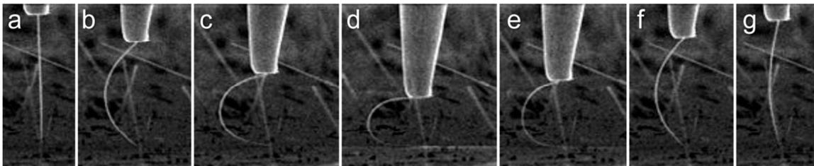
**Figure S6.** SEM images showing U-shape bending (a-d) and complete recovery (e-g) of a Au NW as the Au NW is pushed against a solid surface.
