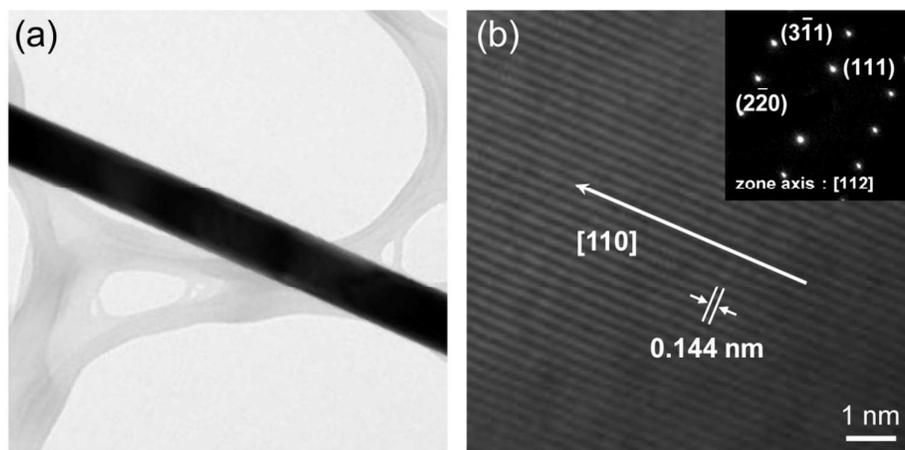
**Figure S3.** (a) TEM image, (b) HRTEM image and selected area electron diffraction (SAED) pattern of a Au NW, indicating that the Au NW is single-crystalline without twins or defects.
