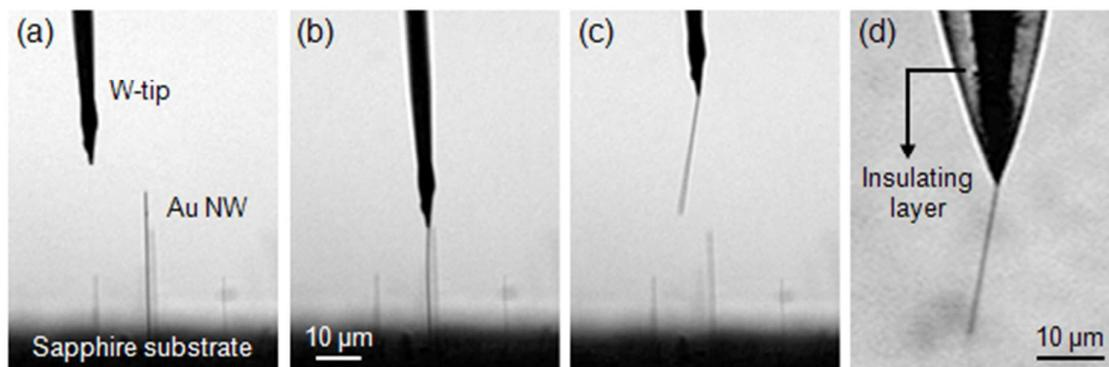
**Figure S2.** Optical images of the fabrication process of a Au NW nanoinjector.
